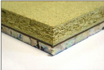
Trim Defender 35 should be laid directly onto the joists in a broken bond pattern with all joints glued and perimeters sealed using 37mm x 10mm Perimeter isolation tape.
