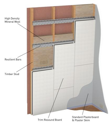
Manufactured in an easy to handle size panel (1200mm x 600mm) and with an innovative self-adhesive jointing system new Trim Resound Board can be easily installed with no need for adhesive.
