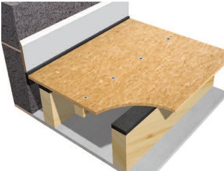
This is a very cost effective way of reducing impact noise in a conventional timber joisted floor. The Impactafoam self adhesive strips are supplied in coil form and are simply applied to the top of the joists providing a resilient seating for the boards. The floor is installed by positioning 50 x 50mm timber battens directly underneath the floor boarding, and centrally between the joists, running parallel to them.
