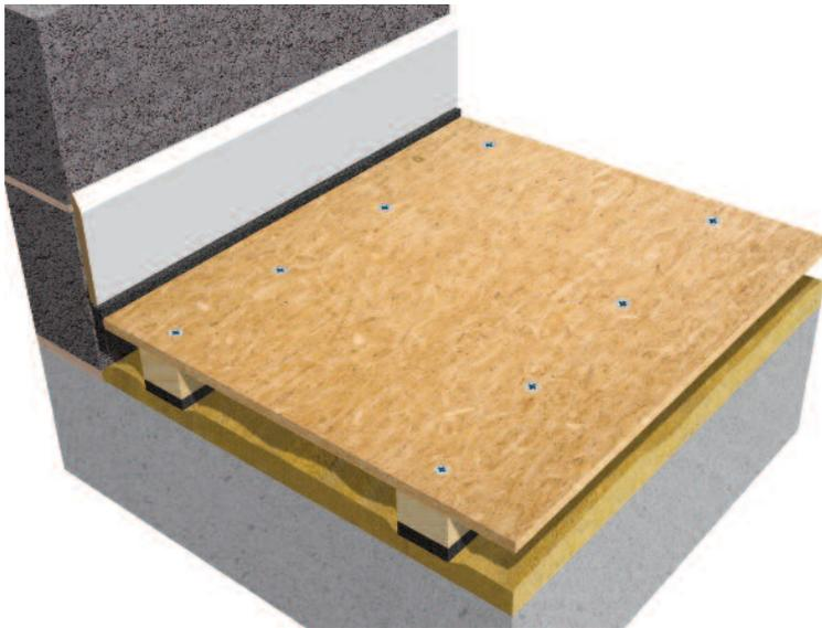
Impactafoam may also be used as part of a raft floor construction on top of a concrete base. Self adhesive strips are applied to 50x50mm timber battens and laid on top of a 13mm thick 36kg/m<sup>3</sup> insulation quilt over the concrete floor. Boards or sheets are then fixed to the battens giving a floating raft layer. The chipboard should be isolated from the perimeter walls using strips of Impactafoam.
