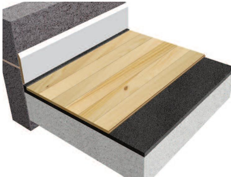
This is an ideal and cost effective method of reducing impact noise caused by footfall or the movement of furniture on a timber or laminate surface. Impactafoam is simply rolled out onto the structural floor and should return up all perimeter walls or columns to stop sound bridging. The laminate floor is laid on top, and should butt up to the Impactafoam at the perimeters. Any overlap should be cut away with a trimming knife. This will completely insulate the laminate floor from the structure.
